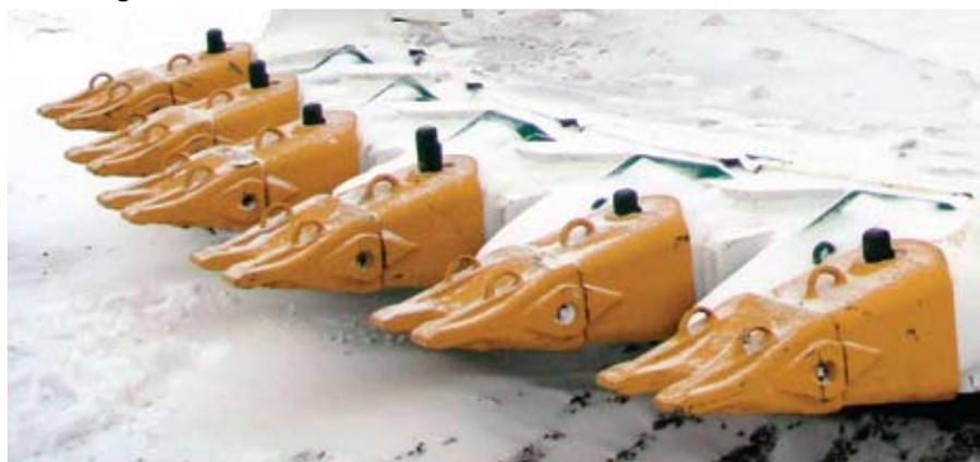
sling for use with a service crane. And once installed, the new tips, constructed of DH3 alloy, are designed to outlast tips constructed of other materials.
